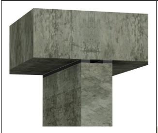
Remove any debris and dust in the opening.
