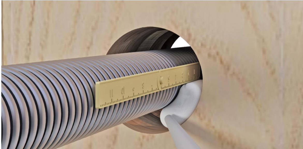
Schematic diagram for correct measurement of sealant depth.
