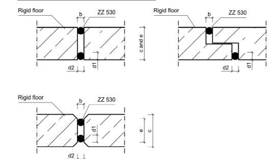
Considering the minimum overall seal depth (150 mm) Fire Protection Joint Seal ZZ 530 need not to be installed flush with the surface in case of rigid floors thicker than 150 mm. All dimensions in mm
